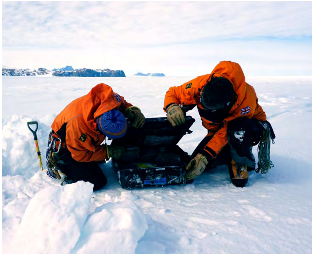
Top right: Dr Stevens and Professor Willis peer into an enclosure containing a GPS receiver, batteries, and a charge controller after digging the enclosure out from beneath two years' worth of snow accumulation on the ice shelf (Photo: M. Chambers (BAS)).
